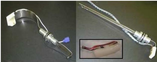
Fig. 6. Force and ischemia sensing Deaver retractor (left) and custom Balfour retractor (right) for open abdominal surgery.
