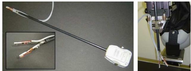
Fig. 11. Instrumented grasper fingers attached to robotic tool for augmenting available information during robotic surgery (left), closeup of the fingers (inset), sensing grasper on Intuitive Surgical's da Vinci robot.
