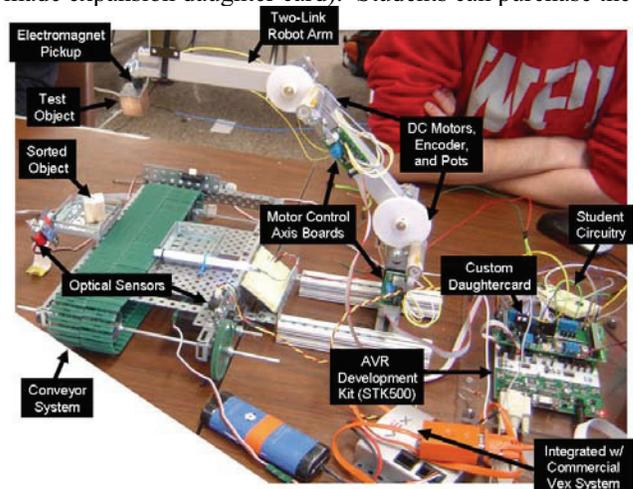
Figure 1: Prototype EduArm system including the 2-Link arm with DC motors, encoders, potentiometers, gear trains, magnetic gripper, sensors, control circuitry, and microcontroller.
