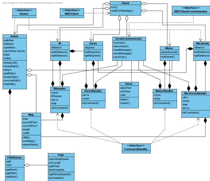
Figure 3: UML representation of the Application Programming Interface (API) developed by RBE 3002 students using the software framework.
