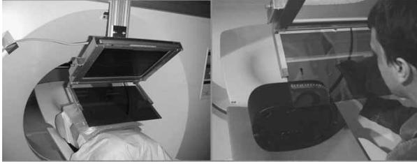
Figure 11. Phantom experiments on a male mannequin (left) and a tissue-equivalent commercial abdominal intervention phantom (right).
