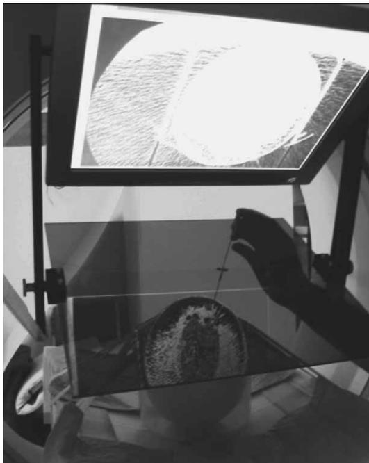
Figure 2. Physician's perspective: the overlay image in the mirror appears to be floating inside the subject while the physician manipulates the needle behind the mirror. (Phantom experiment on a honeydew melon.)
