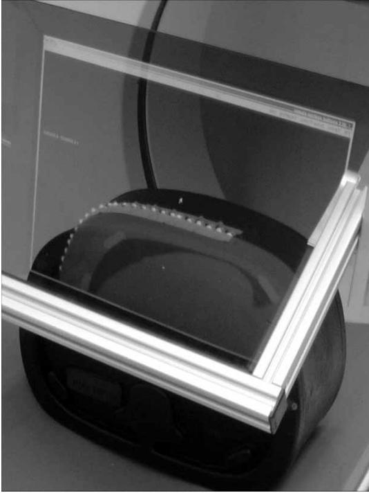
Figure 3. IZI biopsy strip fiducial as seen both on the subject and in the overlay image (abdominal phantom experiment).
