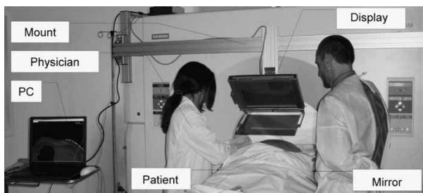
Figure 5. Image overlay system that renders the image in the outer transverse laser plane of the CT scanner. The patient is conveniently accessible for multiple physicians who share the same view.
