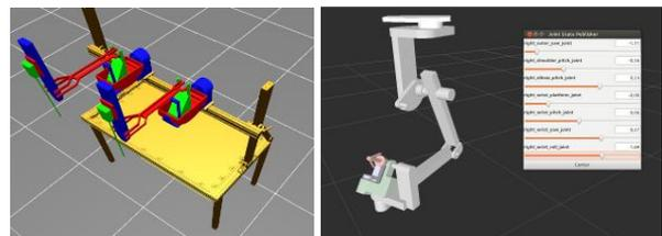
Fig. 2: Kinematic simulation coupled to hardware through ROS. PSMs (left) and MTM with slider control (right).
