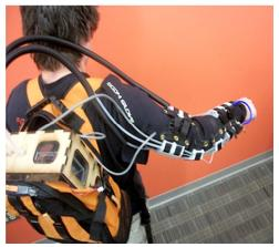
Figure 1. ExoMuscular Orthotic: User wears soft robotic brace with sensor wires and
