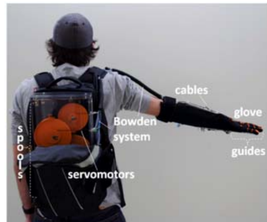
Figure 1. Prototype assembly: user wears the flexible glove with pairs of cables for each finger running through guide tubes, up the length of the arm, to five motorized spools in a lightweight backpack.
