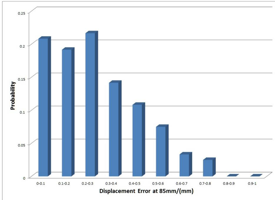
Figure 5 Probability distribution of displacement error. All of the errors are found below 0.8mm
