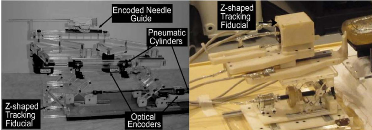
Figure 1 Passive fiducial modules mounted on the needle insertion robots. A system developed by Tokuda et al.(left)<sup>13</sup>, Needle insertion robot developed by Su et al.(right)<sup>5</sup>
