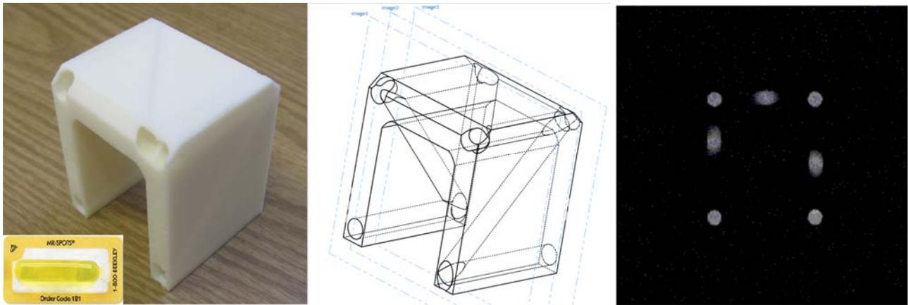
Figure 2 The fiducial tracking module Z-frame(left), CAD model of Z-frame(middle), Z-frame MR image(right) and Beekley fiducial tubes(lower left)
