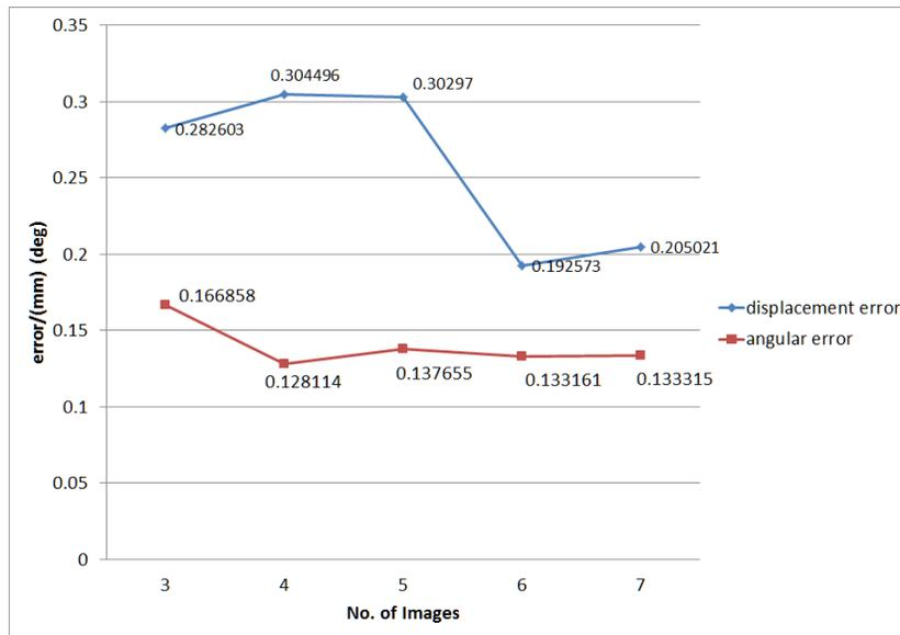
Figure 6 Accuracy comparison between different no. of images evenly distributed in the acquisition volume.
