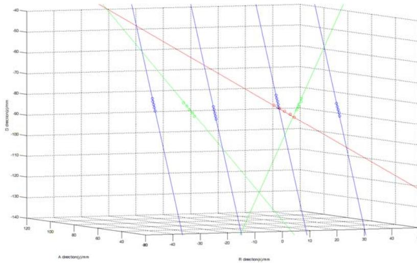
Figure 4 Matlab plot of the spacial pose of the Z-frame by using 5 images. The circle represent the located fiducial centroids in each image, the blue line represent the 4 horizontal fiducial tubes, the green lines represent the angles tubes on the sides, and the red line represents the angled tube on the top surface.
