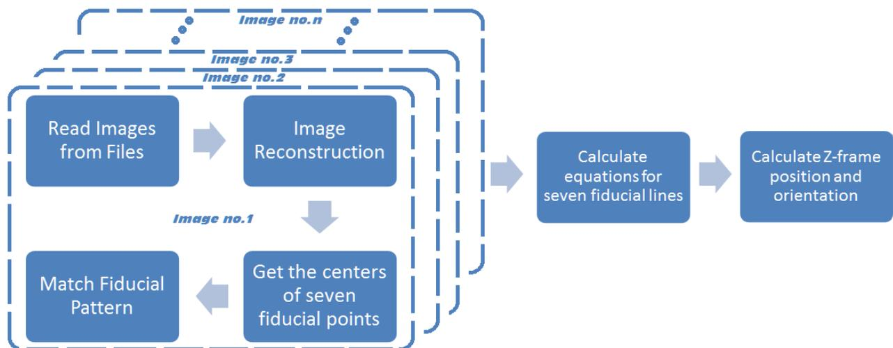
Figure 3 Fiducial Detection and Localization Algorithm
