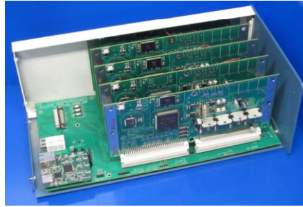
Figure 4. Robot controller's motor driver that contains five piezoelectric driver boards. The custom control system resides in the shielded robot controller enclosure.
