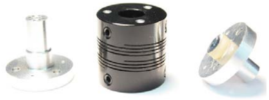
Figure 5: Components of the sensor prototype with fiber guide (left),flexure (center) and cover plate with spherical mirror (right).
