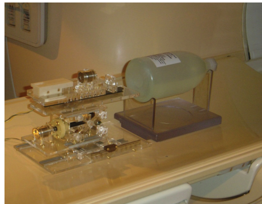
Fig. 1. The prototype robot in the bore of a 3T MRI scanner with a MRI-compatible phantom.
